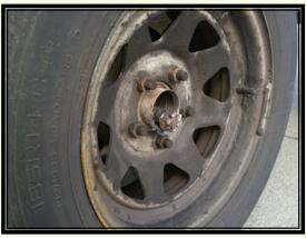
We pulled over into a lane which had been closed due to road works further which gave us plenty of room to fix the trailer. We were prepared with spare bearings, but the damage was a little more widespread. A quick ring around found the required parts, and Greg went to work with angle grinder to repair the damaged axle and replace the bearing.
